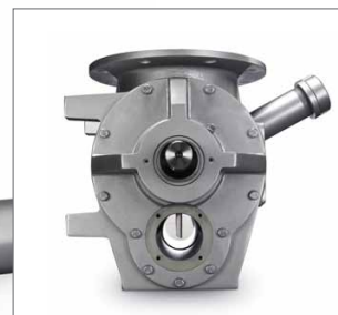
The BT Series valves ensure optimal bulk density and throughput of hard-to-convey material; a return-side vent vents leaked air, maximizing air flow through the rotor, improving material flow.
