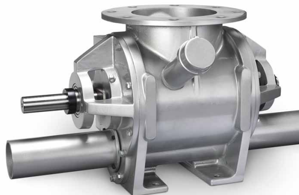
The BT Series valves ensure optimal bulk density and throughput of hard-to-convey material; a return-side vent vents leaked air, maximizing air flow through the rotor, improving material flow.
