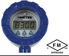
The DT-8300EX is designed for use in process industries, where vibration, inclement weather, and corrosive atmospheres are present. The electronics are enclosed in copper-free, epoxy coated, aluminum housings. The housing is FM explosion proof certified and meets NEMA 4X and IP68 rating standards.
