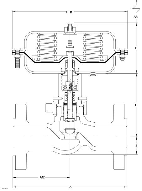
Figure 4. Fisher D3 Control Valve with Size 30 Actuator and NPS 2 Flanged Valve Body (Spring-to-Open Configuration)
