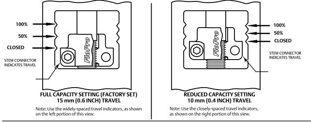
Note: See Fisher Catalog 12 for flow coefficients. Full capacity coefficients are shown as 100 percent valve opening. Reduced capacity coefficients are shown as 60 percent valve opening.
