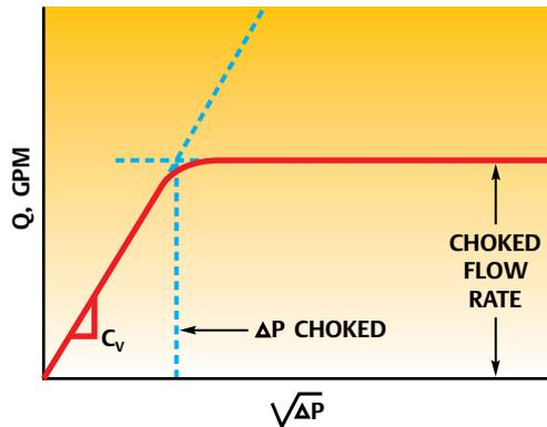
Basic valve sizing equations imply that, for a given valve, flow should continually increase by simply increasing the pressure differential across the valve. In reality, the relationship given by these equations holds true for only a limited range. As the pressure differential is increased, a point is reached where the flow increase stops. This condition of limited maximum flow is known as choked flow.
