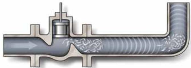
**Throttling across the control valve generates high turbulence. Turbulence will eventually decrease but the acoustic pressure field will persist.**
