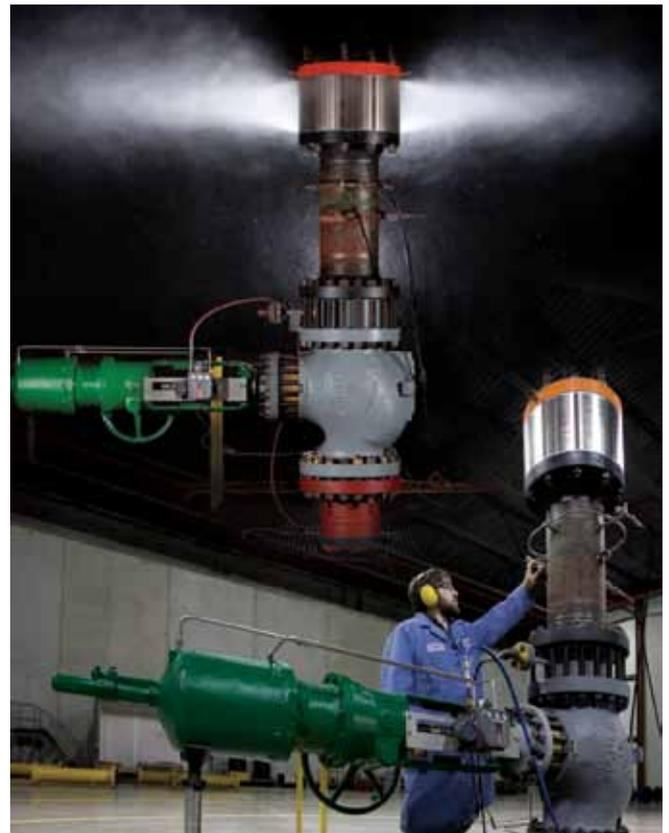
*Noise testing of an NPS 12 vent diffuser.*
