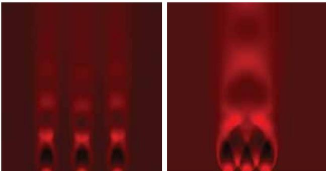
**Computational fluid dynamics show jet independence from three properly spaced holes (left). The same three holes spaced too closely (right) show jet interaction, which leads to additional noise. Being able to predict and control jet interaction can reduce the noise produced by up to 40 dBA.**
