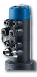
The T.VIS<sup>®</sup> P-1 / P-20 is a compact position controller for pneumatic valves. By specifying a setpoint (4-20 mA), transferred e.g. by the PLC, the process valve can be brought to any position. The position is detected by a position sensor with a resolution of 0.01 mm and adjusted by 2 integrated solenoid valves.
