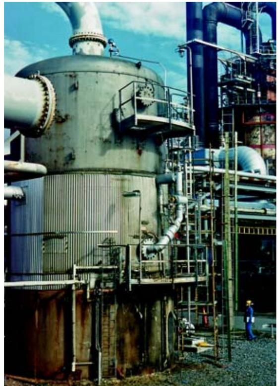
*The blowdown drum is 28 ft (8.5 m) high but the required measuring range is approximately 9.8 ft (3 m). The tank can be filled to a maximum of 9.8 ft (3 m).*
