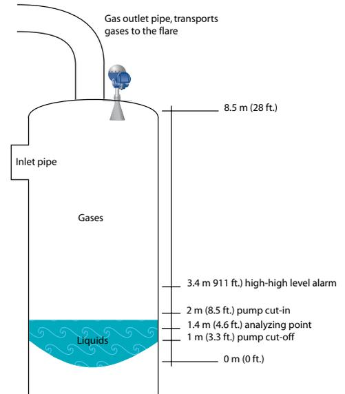
*The blowdown drum at the refinery serves as an accumulator for the refinery process. The Rosemount 5600 measures level and communicates the measurement to the DCS.*
