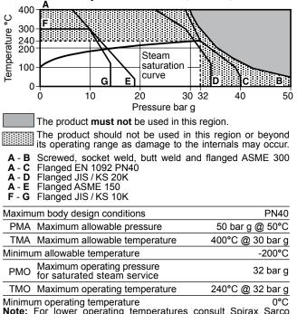
Minimum operating temperature 0°C Note: For lower operating temperatures consult Spirax Sarco Designed for a maximum cold hydraulic test pressure of 75 bar g
