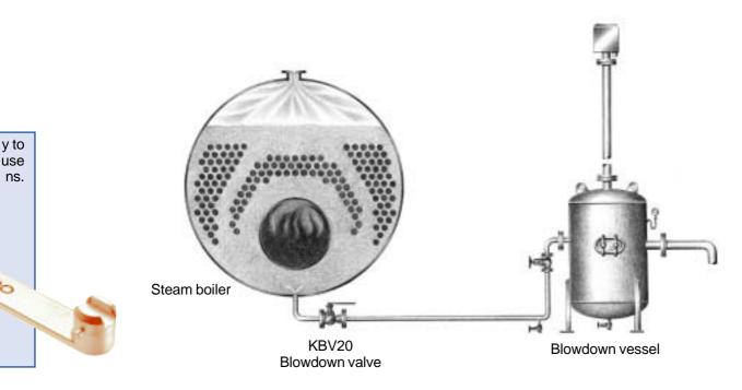
Quarter turn movement from fully closed to fully open ensures correct 'quick burst' operation.
