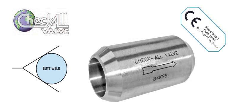
The **Butt Weld (B4, B8)** check valve is a one piece body machined from bar stock, eliminating porosity concerns and providing uniform density for more consistent welds. Made to ASME/ANSI B16.25 for schedule 40 pipe (B4), or schedule 80 pipe (B8) it carries rugged, dependable Check-All® trim with a wide variety of seat materials and cracking pressures to choose from. The Butt Weld valve can also be used as a low pressure relief valve or vacuum breaker by using the desired spring settings.
