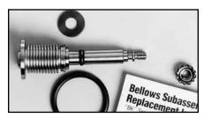
Kits include welded subassembly (stem, bellows, weld ring), piston and stem O-rings, lock nut, washer, and instructions. The ordering number specifies stainless steel **(SS)** for stainless steel and brass valves. For alloy 400 valve kits, replace **SS** with **M**.
