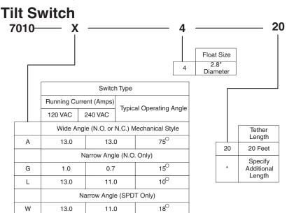
Note - Additional length wire is spliced to existing float wire. Special epoxy heat shrink tube is used to assure watertight seal.
